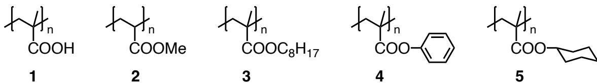
In reference to 2, all other polymers are disubstituted at the main chain carbon, which generally leads to a rigidification of the polymer chain. In brackets are additional factors that further reduce chain mobility and increase  $T_g$  (exception is polymer 3, where the flexible substituent overcompensates the effect of the disubstitution, leading to an overall reduced  $T_g$ ).
